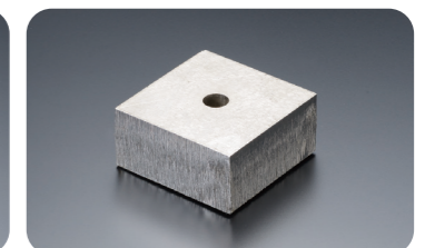
28mm thick separation cutting
