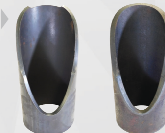
TOKYO SKYTREE Welding preparation (Upper part)
