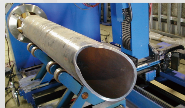
Cutting with AWS Intersecting angle of 37 degrees
