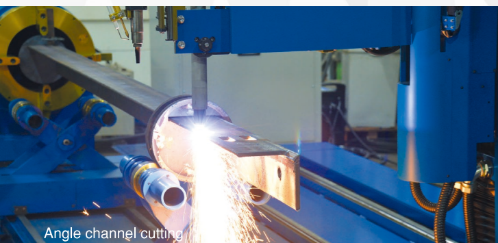
Angle channel cutting
